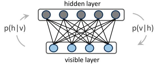
Fig. 3. Graphical representation of a Restricted Boltzmann Machine.
