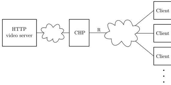
Fig. 1. Reference scenario: the Cognitive HTTP Proxy (CHP) implements the RM and VAC mechanisms to manage the rates of the active video flows across the bottleneck link of capacity  $R$  [bit/s].
