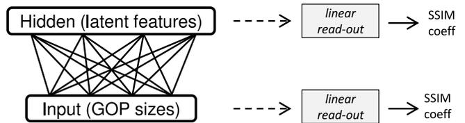
Fig. 4. Scheme of the proposed learning framework, on which unsupervised feature extraction (left) is followed by supervised linear read-out (right).
