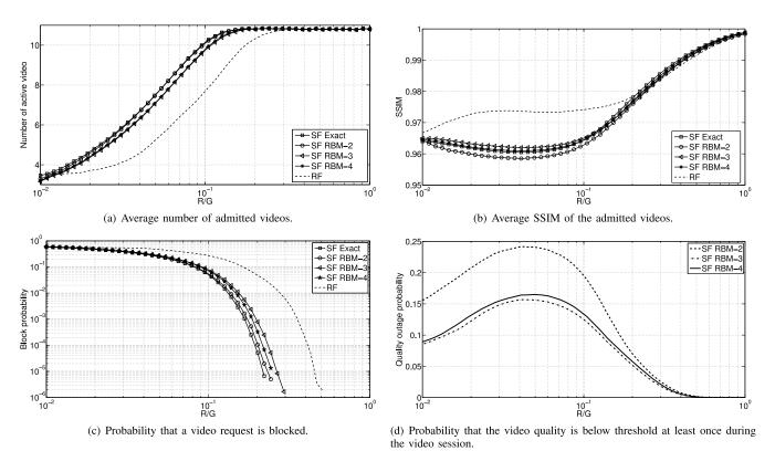
Fig. 8. Performance comparison of our proposed algorithms RF and SF when varying the channel capacity, where SF-Exact is the result based on the exact SSIM curve, while SF-RBM-n is based on the n-degree polynomial estimation given by the RBM model.
