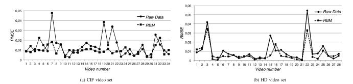
Fig. 5. Root Mean Squared Error (RMSE) of the estimated SSIM-rate curve for each video in the CIF video test set (a) and HD video test set (b), with n = 4. Polynomial coefficients estimation is given by applying a linear classifier on raw input data (circle markers) or on the hidden layer of the RBM (square markers).
