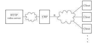
Fig. 1. Reference scenario: the Cognitive HTTP Proxy (CHP) implements the RM and VAC mechanisms to manage the rates of the active video flows across the bottleneck link of capacity R [bit/s].
