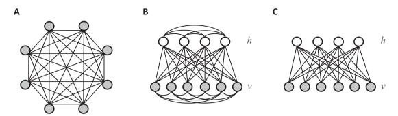
FIG. 1. Graphical representation of several recurrent neural network architectures. (A) Hopfield network, which is a fully connected graph. (B) Boltzmann machine, which is a fully connected graph with two separate sets of units: the visible neurons v are used to perceive input patterns, while the hidden neurons h capture the statistical structure observed in the data. (C) Restricted Boltzmann machine, where intra-layer connections are removed in order to form a bipartite graph.
