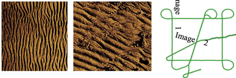
Fig. 1 Example of an apparent shift in the orientation of the sand ripple as a result of an AUV maneuver. Left panel: Image 1, heading 89.8deg. Middle panel: Image 2, heading 15.6deg. Right panel: Track of the AUV
